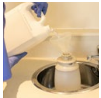
STEP 12 Rinse the water bottle with distilled water
