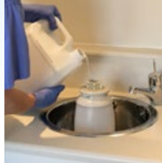
STEP 3 Rinse the water bottle with distilled water
