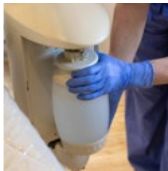
STEP 10 Remove the water bottle after treatment
