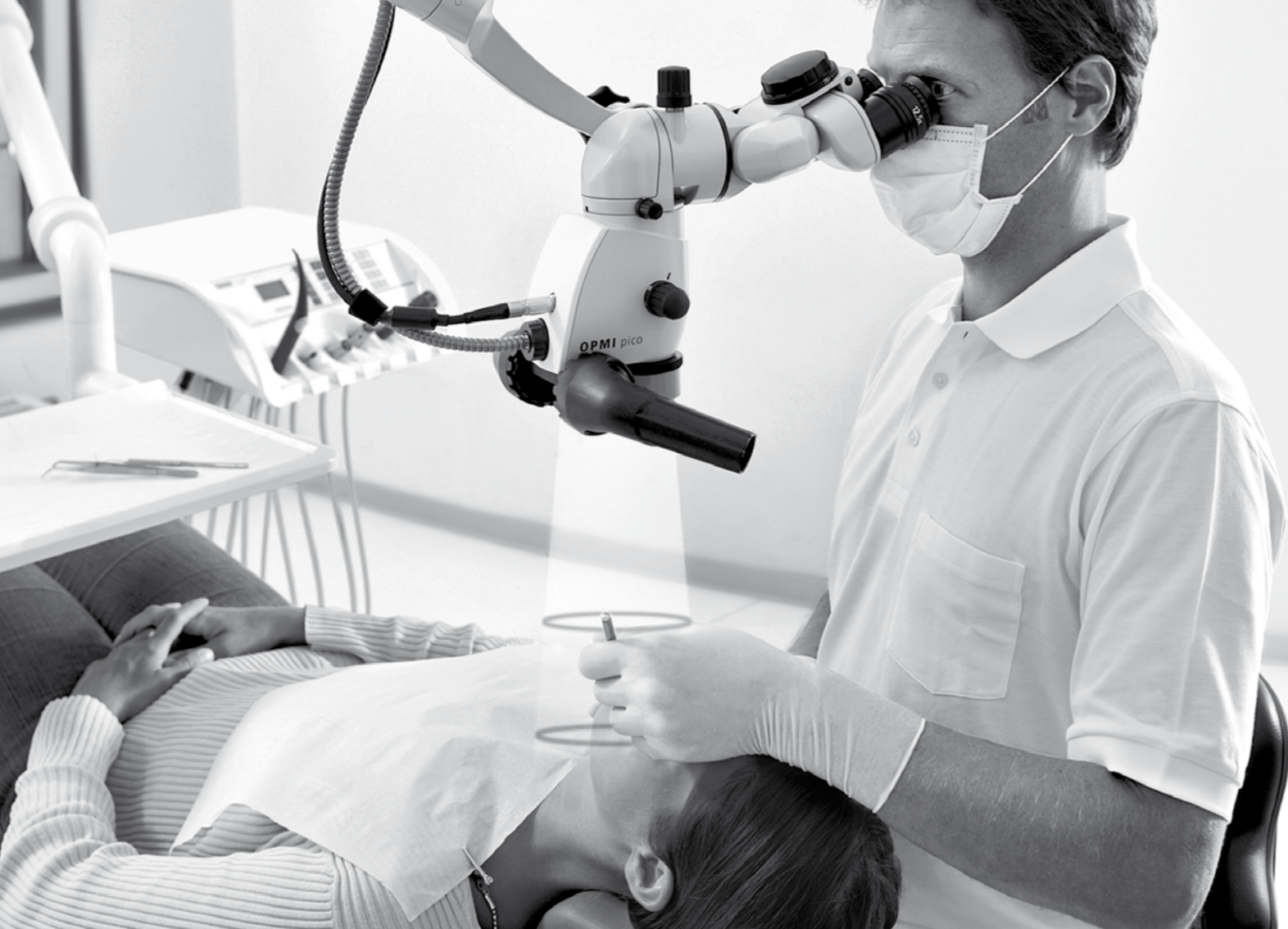
Figure 1.3: Using Varioskop 100 of OPMI pico the dentist can focus continuously, for example, from the incisors to the molars in the patient's oral cavity without changing the position of the OPMI. The height of OPMI pico can be set in a range from 200 to 300 mm above the patient's oral cavity allowing adaptation to the personal ergonomic needs of the dentist.
