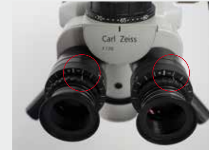
Figure 1.12b Viewing without eyeglasses: set dioptre correction according to your correction value of the eye (e.g. -1)
