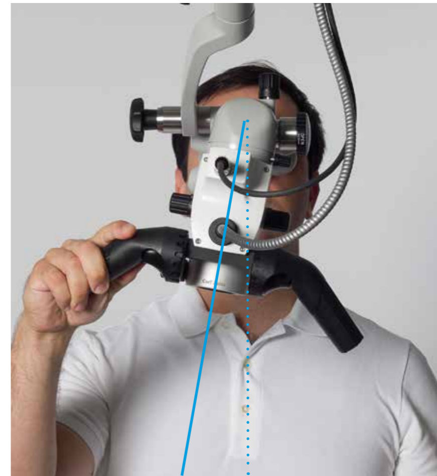
Figure 1.20: The MORA interface allows the OPMI to be tilted to the left or right. The eyepieces retain their horizontal position, so that the dentist has a straight, ergonomic seating position when looking into the OPMI.
