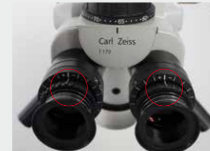
Figure 1.12d Viewing with eyeglasses: set dioptre setting ring on the OPMI to 0 dioptres
