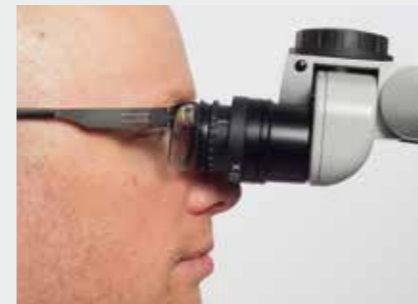
Figure 1.12c Viewing with eyeglasses: screw in the eyecups all the way (no silver ring visible)
