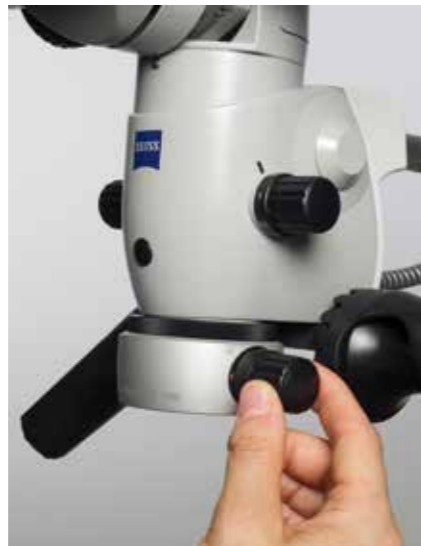
Figure 1.19a: The Varioskop 100 of S100 / OPMI pico allows focussing in the range from 200 - 300 mm by turning the focus knob manually.
